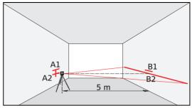
Then place the instrument at the same elevation as close as possible to wall A and again mark the horizontal laser line or the laser dot on wall A (-> A2) . Rotate the instrument by  $180^{\circ}$  again and mark the laser on wall B (-> B2). Measure the distances of the marked points A1-A2 and B1-B2. Calculate the difference of the two measurements. If the difference does not exceed 2 mm, then the Leica Lino is within tolerance.
